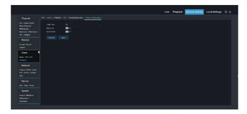
Picture 7-9 Occlusion Detection setting interface
