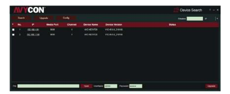
Config: Double-click the selected camera in the search page, turn to the Config page to reboot the camera, change passwords, and reset the camera.
